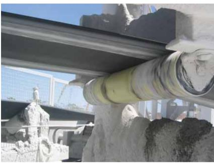
A changeover from steel can conveyor idlers to YeloRoll PVC idlers at a Washington underground zinc mine provided benefits ranging from higher system availability to improved worker safety.
