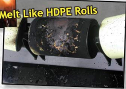
HDPE (Polyethylene) melts and smokes creating fires, damaging belts and bringing production to a stop.
