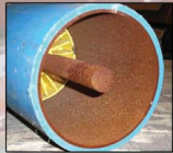
HDPE (Polyethylene) Sleeved Metal Can Roll (belts slide and mistrack)
